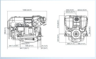
Dimensions may differ according to engine types and are not for installations
